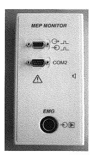
The Trig in/out and COM2 connector are available on the front side of the MEP Monitor.
